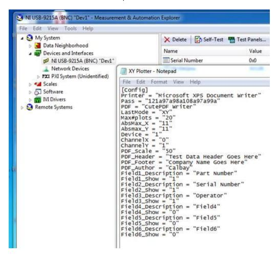
To edit the XY Plotter Device name, open the XY Plotter config file which is located in the XY plotter folder on the drive you saved it to when installing. The config file is shown at the bottom of the list below.
