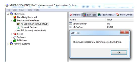
If, as shown above the driver has successfully communicated with the device but when you run the plotter software the cursor still does not move, there is likely to be a problem with the device name. This can occur if you have more than one DAQ card in your computer. You will need to set the XY plotter device name to the same as the one shown in MAX. An example is shown below.
