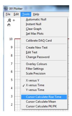
The Software can perform calculations on the trace data once the run has been stopped. Select the button to enable this function. Once the calculation type is selected from the pull down menu, cursor bars will appear on the trace. Move the cursors to the area of interest and the result will be shown on the lower bar.
