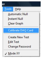
The DAQ card integrity can be checked by using the Calibration routine, this can be run by selecting **Tools – Calibrate DAQ Card**
