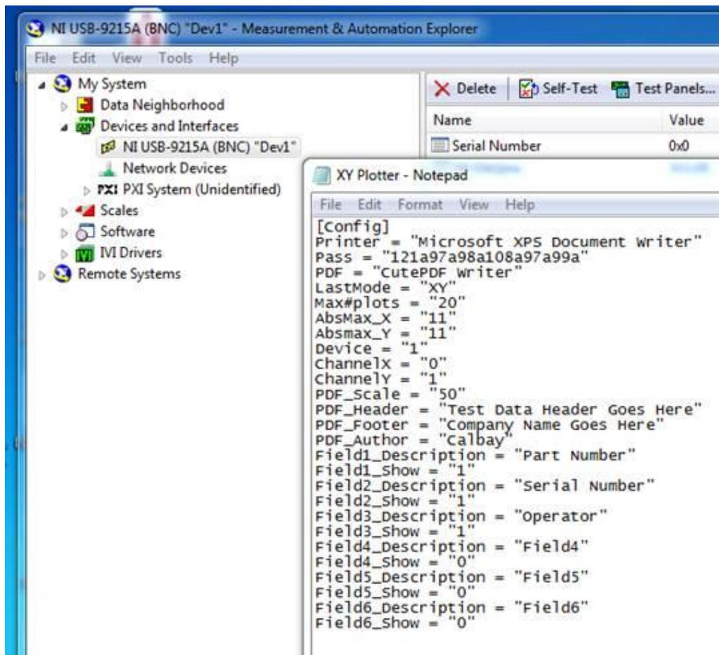
To edit the XY Plotter Device name, open the XY Plotter config file which is located in the XY plotter folder on the drive you saved it to when installing. The config file is shown at the bottom of the list below.
