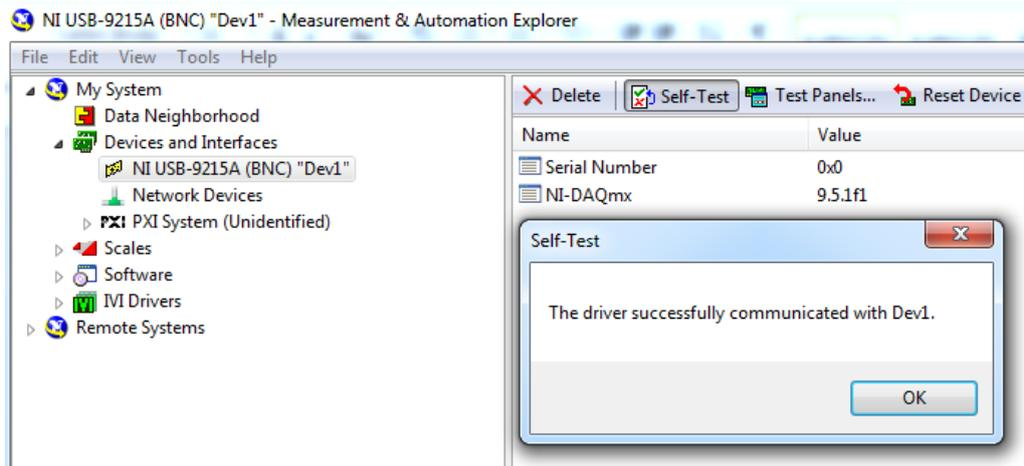
If, as shown above the driver has successfully communicated with the device but when you run the plotter software the cursor still does not move, there is likely to be a problem with the device name. This can occur if you have more than one DAQ card in your computer. You will need to set the XY plotter device name to the same as the one shown in MAX. An example is shown below.
